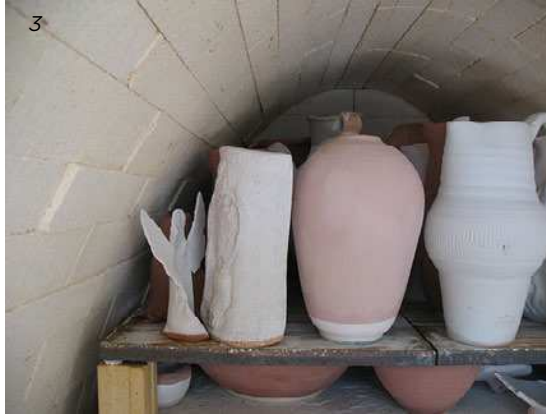
These clay pots have been dried and they have just been loaded into a kiln to be fired.
