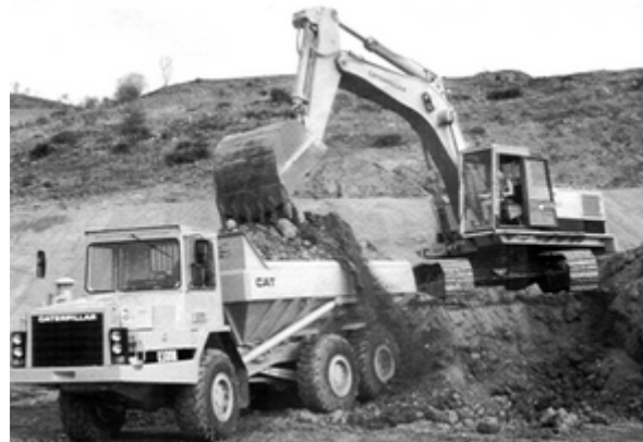
Figure 5.4: Backactor loading tip truck
